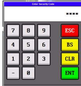
Enter the security code and press the **ENT** button to display the machine's main monitoring screen. The security code will be the machine's serial number (2469 or 2470).
